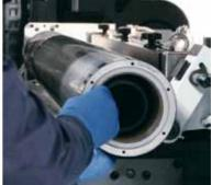
The patented Thermilox® system is applicable to EB and UV flexo presses in order to guarantee the accurate and continuous control of ink temperature during the print run.
